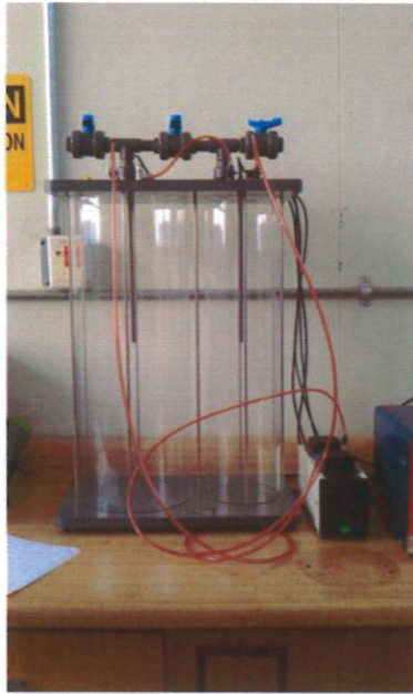
Figure 2 Rigid vessels with base and top-plates and associated valves and tubing
