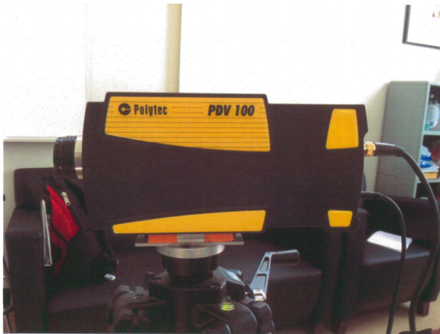
Figure 2 Polytec PDV 100 Digital Vibrometer mounted on tripod
