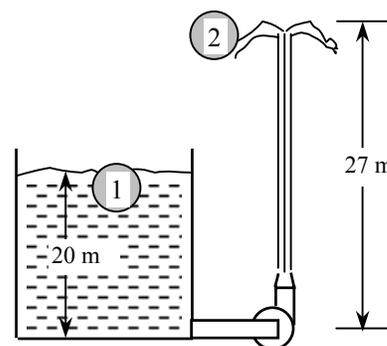
Therefore, the pump must supply a minimum pressure rise of 68.7 kPa.
