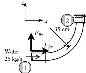
**6-23** An 180° elbow forces the flow to make a U-turn and discharges it to the atmosphere at a specified rate. The gage pressure at the inlet of the elbow and the anchoring force needed to hold the elbow in place are to be determined. √
