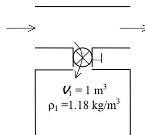
**5-11** The ventilating fan of the bathroom of a building runs continuously. The mass of air “vented out” per day is to be determined.
