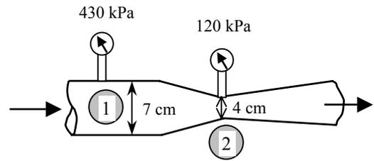
The flow rate for the given case can be determined by substituting the given values into this relation to be
