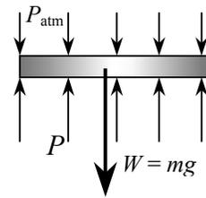
**3-118** The gage pressure in a pressure cooker is maintained constant at 100 kPa by a petcock. The mass of the petcock is to be determined.
