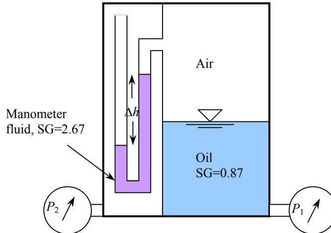
**3-135** An oil pipeline and a rigid air tank are connected to each other by a manometer. The pressure in the pipeline and the change in the level of manometer fluid due to a air temperature drop are to be determined.
