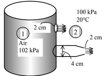
Adding a 2-m long larger diameter lead section will have **no effect** on the flow rate since the flow is frictionless (by using the Bernoulli equation, it can be shown that the velocity in this section increases, but the pressure decreases, and there is a smaller pressure difference to drive the flow through the tap, with zero net effect on the discharge rate).
