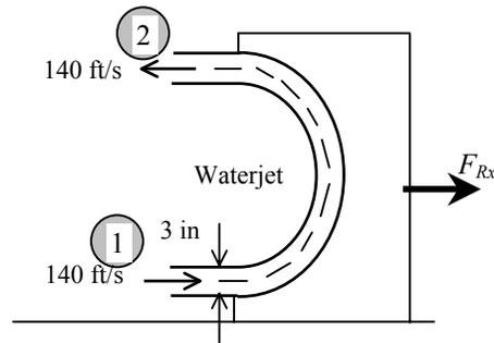
**6-35E** A horizontal water jet strikes a bent plate, which deflects the water by  $135^\circ$  from its original direction. The force required to hold the plate against the water stream is to be determined.
