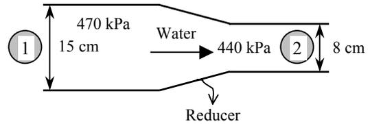
Substituting, the head loss in the reducer is determined to be
