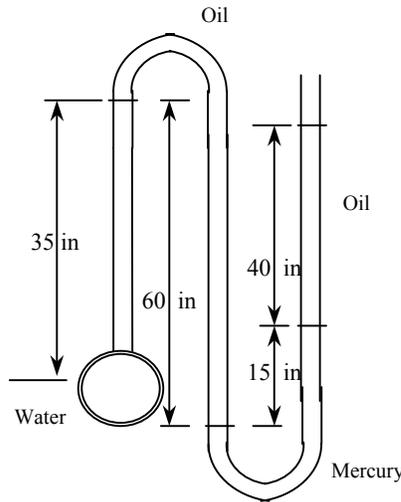
**3-127** The pressure of water flowing through a pipe is measured by an arrangement that involves both a pressure gage and a manometer. For the values given, the pressure in the pipe is to be determined.
