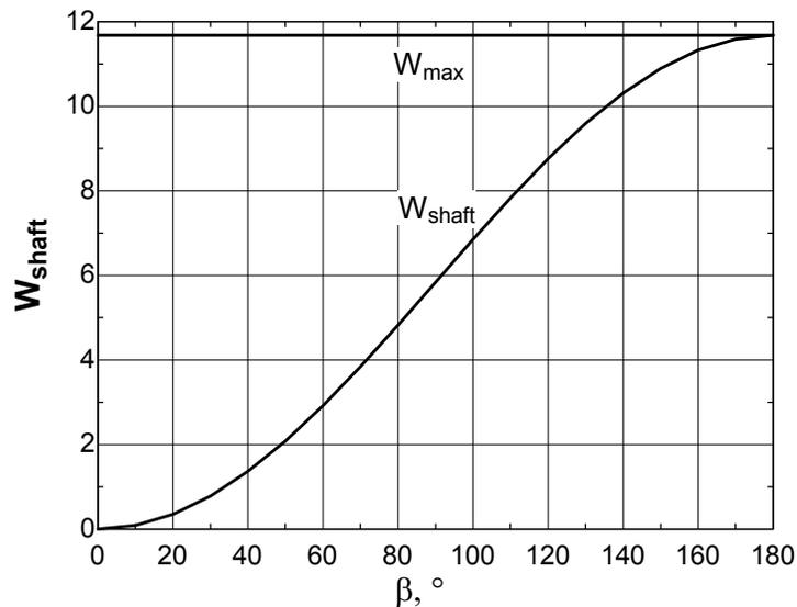
The effectiveness of Pelton wheel for  $\beta = 160^\circ$  is 0.97. Therefore, at this angle, only 3% of power is lost.
