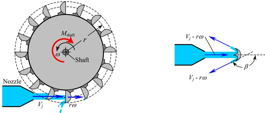
**Assumptions** 1 The flow is uniform and cyclically steady. 2 The water is discharged to the atmosphere, and thus the gage pressure at the nozzle outlet is zero. 3 Generator losses and air drag of rotating components are neglected. 4 The nozzle diameter is small compared to the moment arm, and thus we use average values of radius and velocity at the outlet.
