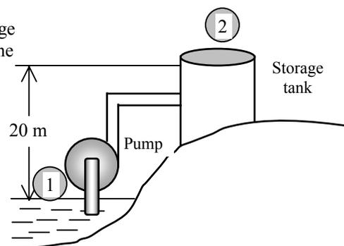
Therefore, the pump must boost the pressure of water by 196 kPa in order to raise its elevation by 20 m.
