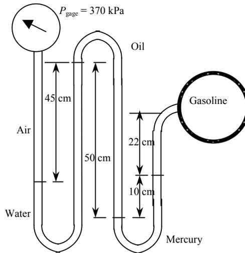
**3-125** A gasoline line is connected to a pressure gage through a double-U manometer. For a given reading of the pressure gage, the gage pressure of the gasoline line is to be determined.
