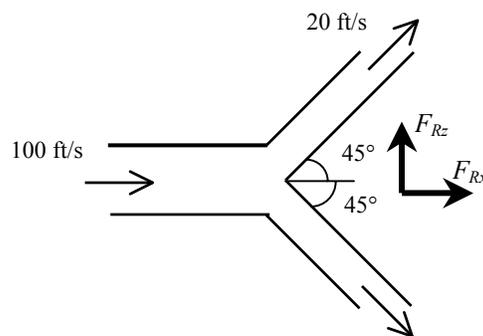
6-30E Problem 6-29E is reconsidered. The effect of splitter angle on the force exerted on the splitter as the half splitter angle varies from 0 to 180° in increments of 10° is to be investigated.
