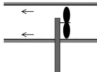
**5-12** A desktop computer is to be cooled by a fan at a high elevation where the air density is low. The mass flow rate of air through the fan and the diameter of the casing for a given velocity are to be determined.
