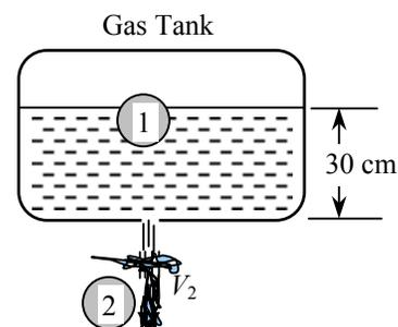
**Discussion** The Bernoulli equation applies along a streamline, and streamlines generally do not make sharp turns. The velocity will be less than 2.43 m/s since the hole is probably sharp-edged and it will cause some head loss.
