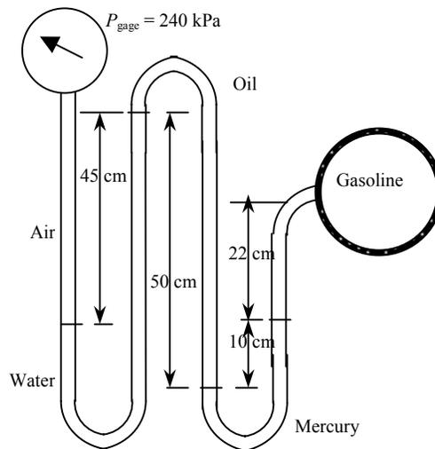
**3-126E** A water pipe is connected to a double-U manometer whose free arm is open to the atmosphere. The absolute pressure at the center of the pipe is to be determined.
