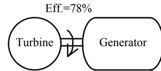
$$\dot{W}_{\text{turbine}} = \eta_{\text{turbine}} \dot{m} g h_{\text{turbine}} = \eta_{\text{turbine}} \rho \dot{V} g h_{\text{turbine}}$$
