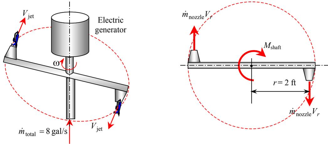
**Assumptions** 1 The flow is uniform and cyclically steady (i.e., steady from a frame of reference rotating with the sprinkler head). 2 The water is discharged to the atmosphere, and thus the gage pressure at the nozzle outlet is zero. 3 The nozzle diameter is small compared to the moment arm, and thus we use average values of radius and velocity at the outlet.
