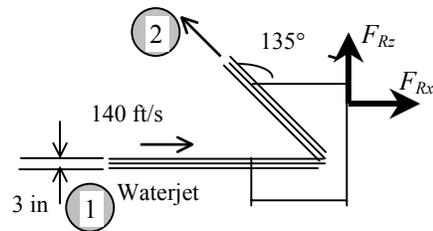
**6-36** Firemen are holding a nozzle at the end of a hose while trying to extinguish a fire. The average water outlet velocity and the resistance force required of the firemen to hold the nozzle are to be determined.
