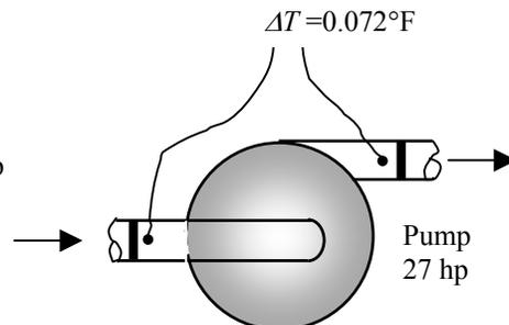
**Discussion** Note that despite the conversion of more than one-third of the mechanical power input into thermal energy, the temperature of water rises by only a small fraction of a degree. Therefore, the temperature rise of a fluid due to frictional heating is usually negligible in heat transfer analysis.
