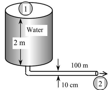
**5-103** Problem 5-102 is reconsidered. The effect of the tank height on the initial discharge velocity of water from the completely filled tank as the tank height varies from 2 to 20 m in increments of 2 m at constant head loss is to be investigated.
