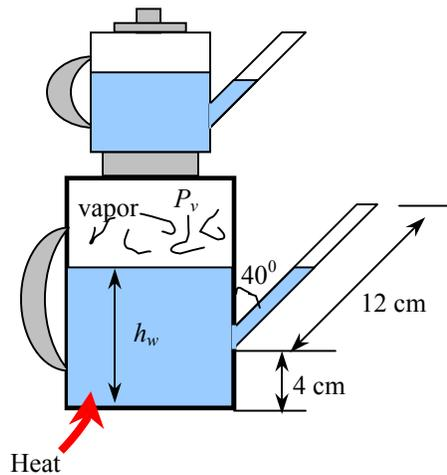
**3-130** The pressure buildup in a teapot may cause the water to overflow through the service tube. The maximum cold-water height to avoid overflow under a specified gage pressure is to be determined by considering the effect of thermal expansion.
