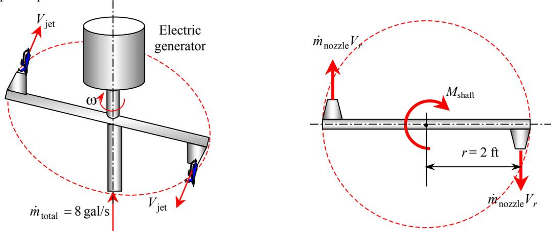
**Assumptions** 1 The flow is cyclically steady (i.e., steady from a frame of reference rotating with the sprinkler head). 2 The water is discharged to the atmosphere, and thus the gage pressure at the nozzle outlet is zero. 3 Generator losses and air drag of rotating components are neglected. 4 The nozzle diameter is small compared to the moment arm, and thus we use average values of radius and velocity at the outlet.
