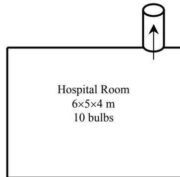
Therefore, the diameter of the duct must be at least 0.16 m to ensure that the air in the room is exchanged completely within 20 min while the mean velocity does not exceed 5 m/s.
