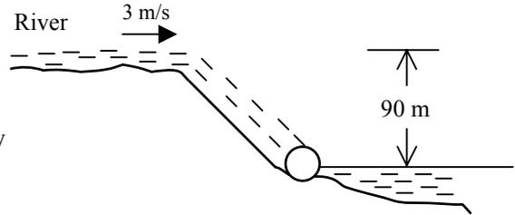
The power generation potential of the river water is obtained by multiplying the total mechanical energy by the mass flow rate,
