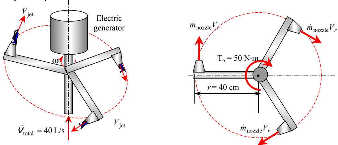
**Assumptions 1** The flow is uniform and cyclically steady (i.e., steady from a frame of reference rotating with the sprinkler head). **2** The water is discharged to the atmosphere, and thus the gage pressure at the nozzle outlet is zero. **3** Air drag of rotating components are neglected. **4** The nozzle diameter is small compared to the moment arm, and thus we use average values of radius and velocity at the outlet.
