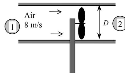
We take points 1 and 2 on the inlet and exit sides of the fan, respectively. Point 1 is sufficiently far from the fan so that  $P_1 = P_{\text{atm}}$  and the flow velocity is negligible ( $V_1 = 0$ ). Also,  $P_2 = P_{\text{atm}}$ . Then the energy equation for this control volume between the points 1 and 2 reduces to
