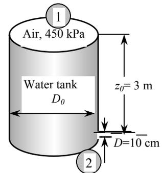
**Discussion** Note that the discharging time is inversely proportional to the square of the orifice diameter. Therefore, the discharging time can be reduced to one-fourth by doubling the diameter of the orifice.
