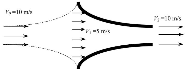
Results:  $V_1 = 5$  m/s,  $V_2 = 10$  m/s,  $m = 12$  kg/s
