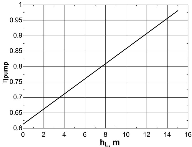
Note that the useful pumping power is used to raise the fluid and to overcome head losses. For a given power input, the pump that overcomes more head loss is more efficient.
