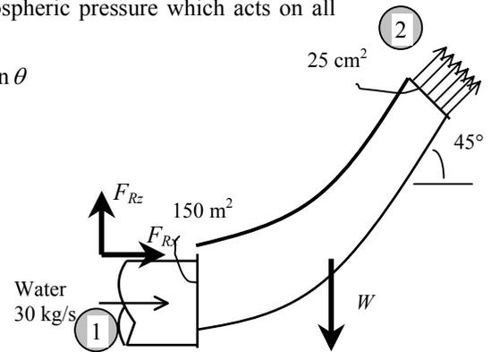
**6-26** A reducing elbow deflects water upwards and discharges it to the atmosphere at a specified rate. The anchoring force needed to hold the elbow in place is to be determined.  $\surd$
