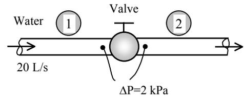
The useful pumping power needed to overcome this head loss is
