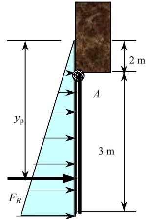
**3-140** A rectangular gate hinged about a horizontal axis along its upper edge is restrained by a fixed ridge at point *B*. The force exerted to the plate by the ridge is to be determined.
