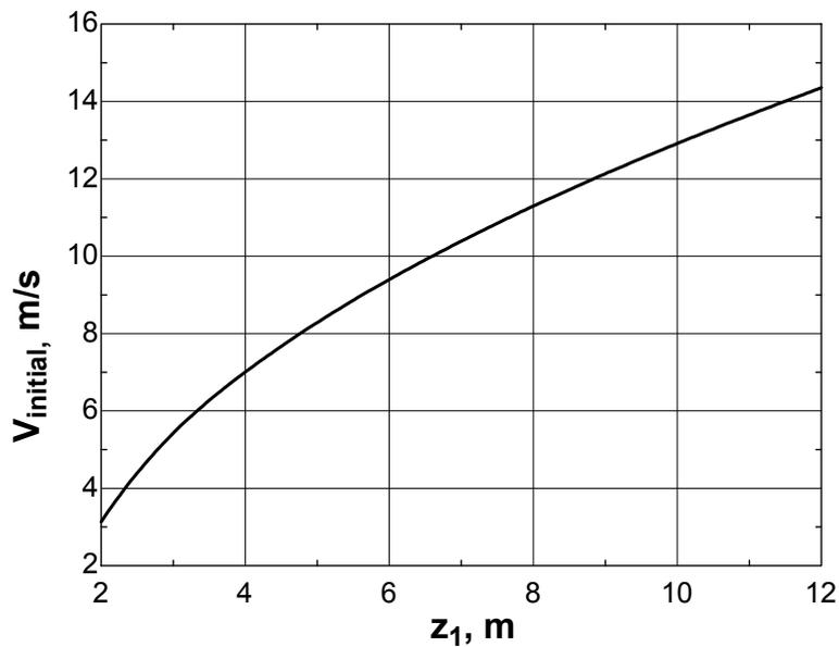
**5-104** A water tank open to the atmosphere is initially filled with water. A sharp-edged orifice at the bottom drains to the atmosphere through a long pipe equipped with a pump with a specified head loss. The required pump head to assure a certain velocity is to be determined.
