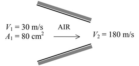
**5-8** Air is expanded and is accelerated as it is heated by a hair dryer of constant diameter. The percent increase in the velocity of air as it flows through the drier is to be determined.
