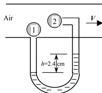
**Discussion** Note that the flow velocity in a pipe or duct can be measured easily by a Pitot-static probe by inserting the probe into the pipe or duct parallel to flow, and reading the differential pressure height. Also note that this is the velocity at the location of the tube. Several readings at several locations in a cross-section may be required to determine the mean flow velocity.
