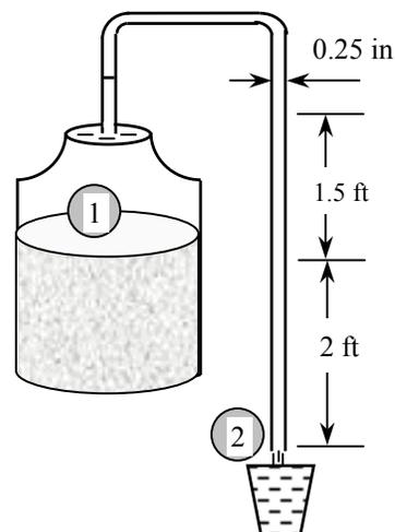
**Discussion** The siphoning time is determined assuming frictionless flow, and thus this is the *minimum time* required. In reality, the time will be longer because of friction between water and the tube surface.
