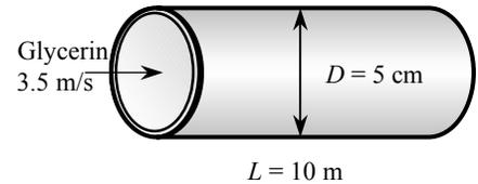
8-47 In Prob. 8-46, the effect of the pipe diameter on the pressure drop for the same constant flow rate is to be investigated by varying the pipe diameter from 1 cm to 10 cm in increments of 1 cm.
