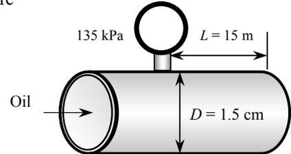
**8-44** Glycerin is flowing through a horizontal pipe which discharges into the atmosphere at a specified flow rate. The absolute pressure at a specified location in the pipe, and the angle  $\theta$  that the pipe must be inclined downwards for the pressure in the entire pipe to be atmospheric pressure are to be determined.
