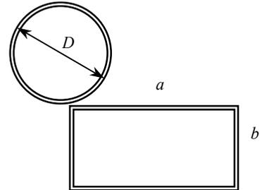
where  $D_h = \frac{4A_c}{p} = \frac{4ab}{2(a+b)} = \frac{2ab}{(a+b)}$  is the hydraulic diameter.
