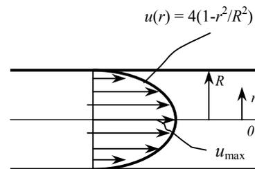
**8-36** The velocity profile in fully developed laminar flow in a circular pipe is given. The average and maximum velocities as well as the flow rate are to be determined.
