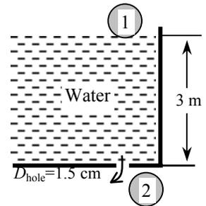
$$\text{Well-rounded entrance: } \dot{V} = \frac{\pi D_{\text{hole}}^2}{4} \sqrt{\frac{2gz_1}{1 + K_L}} = \frac{\pi(0.015 \text{ m})^2}{4} \sqrt{\frac{2(9.81 \text{ m/s}^2)(3 \text{ m})}{1 + 0.03}} = \mathbf{1.34 \times 10^{-3} \text{ m}^3/\text{s}}$$
