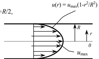
**8-35** The velocity profile in fully developed laminar flow in a circular pipe is given. The average and maximum velocities as well as the flow rate are to be determined.
