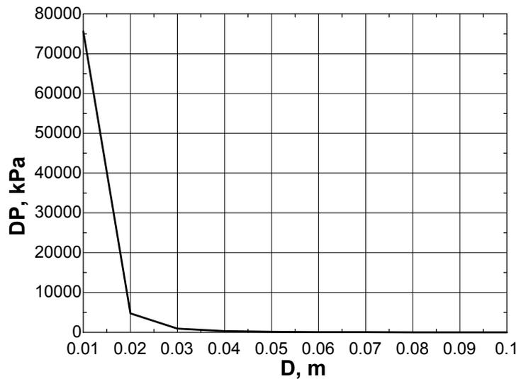
**8-48E** Air is flowing through a square duct made of commercial steel at a specified rate. The pressure drop and head loss per ft of duct are to be determined.
