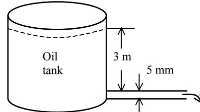
**8-31** The average flow velocity in a pipe is given. The pressure drop, the head loss, and the pumping power are to be determined.  $\surd$
