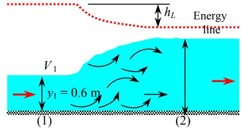
**13-86** Water flowing in a wide channel at a specified depth and flow rate undergoes a hydraulic jump. The mechanical power wasted during this process is to be determined.
