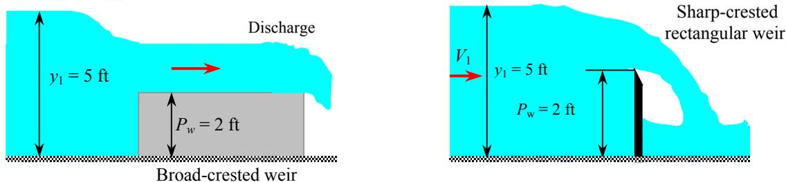
**Assumptions** 1 The flow is steady. 2 The upstream velocity head is negligible. 3 The channel is sufficiently wide so that the end effects are negligible.
