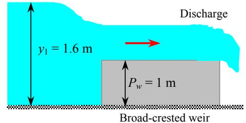
The minimum flow depth above the weir is the critical depth, which is determined from
