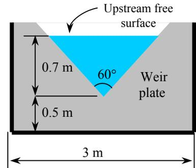
**13-111** The notch angle of a sharp-crested triangular weir used to measure the discharge rate of water from a lake is reduced by half. The percent reduction in the discharge rate is to be determined.
