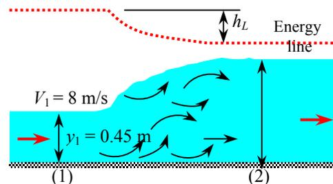
**13-136** The flow depth and average velocity of water after a hydraulic jump together with approach velocity to sluice gate are given. The flow rate per m width, the flow depths before and after the gate, and the energy dissipation ratio are to be determined.
