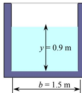
**13-119** The flow of water in a rectangular channel is considered. The effect of bottom slope on the flow rate is to be investigated as the bottom angle varies from 0.5 to 10°.
