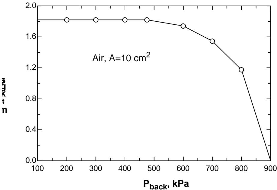
**12-67E** Air enters a converging-diverging nozzle at a specified temperature and pressure with low velocity. The pressure, temperature, velocity, and mass flow rate are to be calculated in the specified test section.
