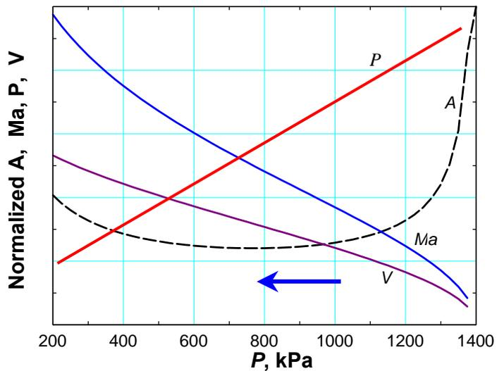
**12-57** For supersonic flow at the inlet, the variation of pressure, velocity, and Mach number along the length of the nozzle are to be sketched for an ideal gas under specified conditions.
