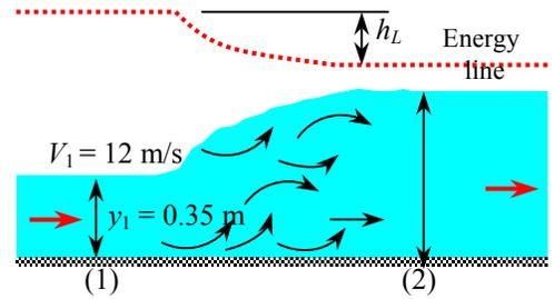
**13-85** The increase in flow depth during a hydraulic jump is given. The velocities and Froude numbers before and after the jump, and the energy dissipation ratio are to be determined.
