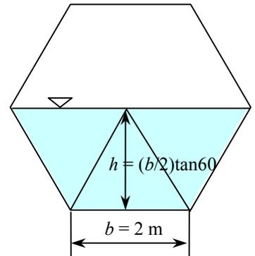
**13-40** Water flows uniformly through a half-full hexagon channel. For a given flow rate, the average velocity and whether the flow is subcritical or supercritical are to be determined.
