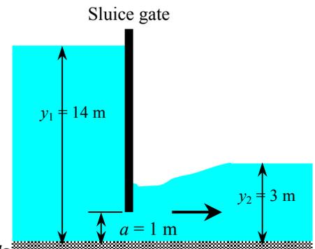
**Discussion** Discharge coefficient is the same as free flow because of small depth ratio after the gate. So, the flow rate would not change if it were not drowned.
