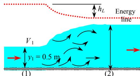
**13-140** The flow rate in an open channel is to be measured using a sharp-crested rectangular weir. For a measured value of flow depth upstream, the flow rate is to be determined.  $\sqrt{EES}$
