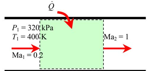
**12-112** Air flowing at a supersonic velocity in a duct is decelerated by heating. The highest temperature air can be heated by heat addition and the rate of heat transfer are to be determined.
