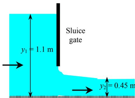
**Assumptions** **1** The flow is steady. **2** The channel is sufficiently wide so that the end effects are negligible. **3** Frictional effects associated with sluice gate are negligible. **4** The channel is horizontal.
