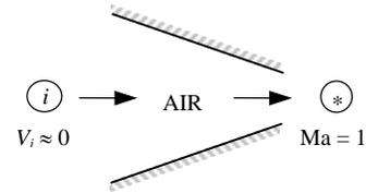
**12-60E** Air enters a nozzle at specified temperature, pressure, and velocity. The exit pressure, exit temperature, and exit-to-inlet area ratio are to be determined for a Mach number of  $Ma = 1$  at the exit.
