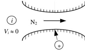
Critical properties are those at a location where the Mach number is  $Ma = 1$ . From Table A-13 at  $Ma = 1$ , we read  $T/T_0 = 0.8333$ ,  $P/P_0 = 0.5283$ , and  $\rho/\rho_0 = 0.6339$ . Then the critical properties become
