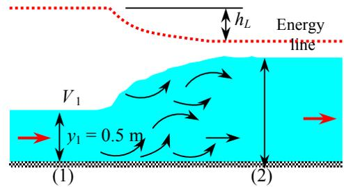
**13-87** The flow depth and average velocity of water after a hydraulic jump are measured. The flow depth and velocity before the jump as well as the fraction of mechanical energy dissipated are to be determined.
