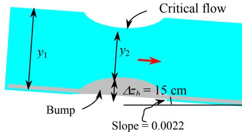
**Assumptions** 1 The flow is steady and uniform. 2 Bottom slope is constant. 3 Roughness coefficient is constant along the channel. 4 The channel is sufficiently wide so that the end effects are negligible. 5 Frictional effects during flow over the bump are negligible.
