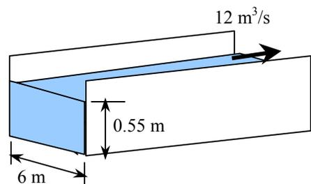
**13-35E** Water flows in a wide rectangular channel. For specified values of flow depth and average velocity, the Froude number, critical depth, and whether the flow is subcritical or supercritical are to be determined.
