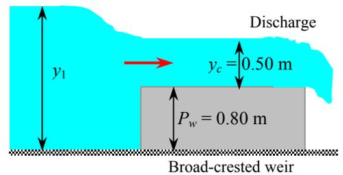
Its solution is  $H = 1.40 \text{ m}$ . Then the flow depth upstream the weir becomes
