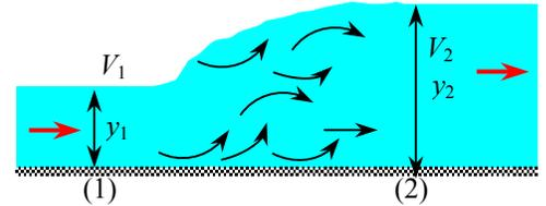
**13-134** A sluice gate with free outflow is used to control the flow rate of water. For specified flow depths, the flow rate per unit width and the downstream flow depth and velocity are to be determined.  $\sqrt{EES}$
