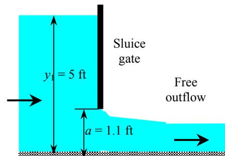
The specific energy of a fluid remains constant during horizontal flow when the frictional effects are negligible,  $E_{s1} = E_{s2}$ . With these approximations, the flow depth past the gate and the Froude number are determined to be
