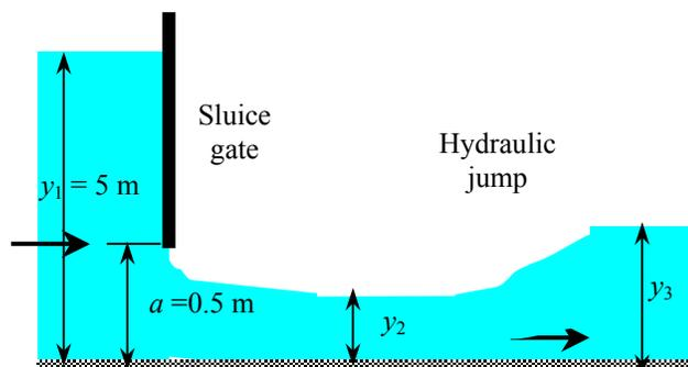
**13-139** Water is discharged from a dam into a wide spillway to reduce the risk of flooding by dissipating a large fraction of mechanical energy via hydraulic jump. For specified flow depths, the velocities before and after the jump, and the mechanical power dissipated per meter width of the spillway are to be determined.
