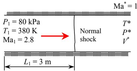
**Assumptions 1** The assumptions associated with Fanno flow (i.e., steady, frictional flow of an ideal gas with constant properties through a constant cross-sectional area adiabatic duct) are valid. **2** The friction factor is constant along the duct.
