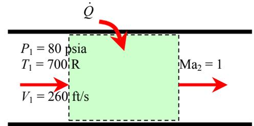
The Rayleigh flow functions corresponding to the inlet and exit Mach numbers are (Table A-15):
