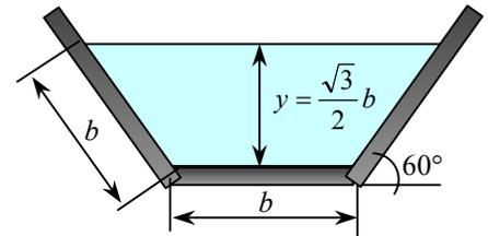
**13-67E** Water is to be transported in a rectangular channel at a specified rate. The dimensions for the best cross-section if the channel is made of unfinished and finished concrete are to be determined.
