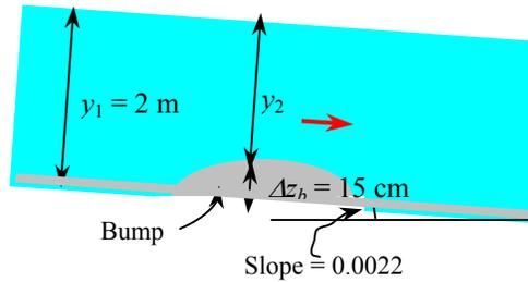
**Assumptions** 1 The flow is steady and uniform. 2 Bottom slope is constant. 3 Roughness coefficient is constant along the channel. 4 The channel is sufficiently wide so that the end effects are negligible. 5 Frictional effects during flow over the bump are negligible.
