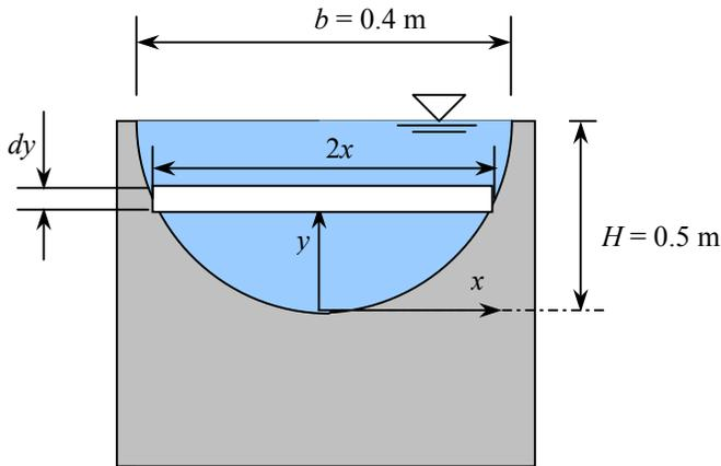
**Analysis** The notch is parabolic with  $y = 0$  at  $x = 0$ , and thus it can be expressed analytically as  $y = Cx^2$ . Using the coordinates of the upper right corner, the value of the constant is determined to be  $C = y/x^2 = H/(b/2)^2 = 4H/b^2 = 4(0.5 \text{ m})/(0.4 \text{ m})^2 = 12.5 \text{ m}^{-1}$ .
