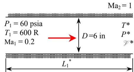
Thus, for the given friction factor, the duct length must be 291 ft for the Mach number to reach  $Ma = 1$  at the duct exit.
