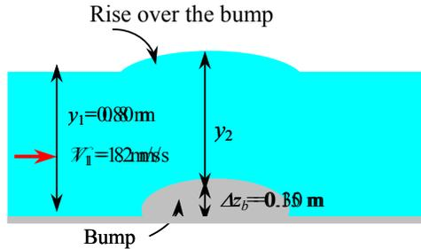
**Assumptions** 1 The flow is steady. 2 Frictional effects are negligible so that there is no dissipation of mechanical energy. 3 The channel is sufficiently wide so that the end effects are negligible.
