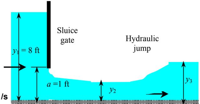
The specific energy of a fluid remains constant during horizontal flow when the frictional effects are negligible,  $E_{s1} = E_{s2}$ . With these approximations, the flow depth past the gate and the Froude number are determined to be
