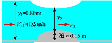
**Assumptions** **1** The flow is steady. **2** Frictional effects are negligible so that there is no dissipation of mechanical energy. **3** The channel is sufficiently wide so that the end effects are negligible.
