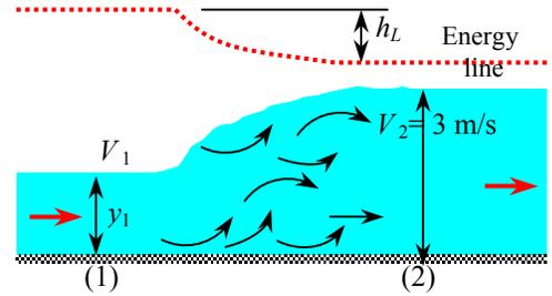
**13-88E** Water at a specified depth and velocity undergoes a hydraulic jump, and dissipates a known fraction of its energy. The flow depth, velocity, and Froude number after the jump and the head loss associated with the jump are to be determined.
