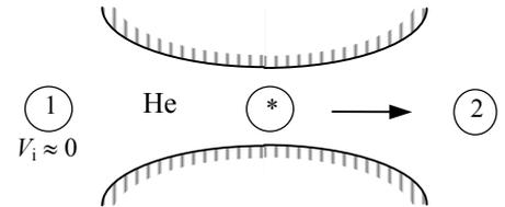
**12-149E** Helium gas is accelerated in a nozzle. For a specified mass flow rate, the throat and exit areas of the nozzle are to be determined for the cases of isentropic and 97% efficient nozzles.
