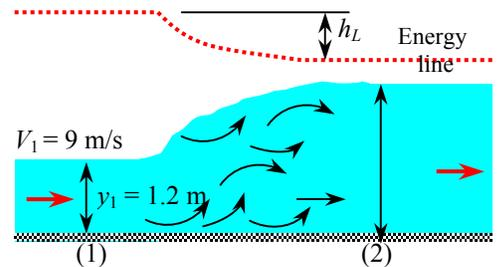
**13-84** Water at a specified depth and velocity undergoes a hydraulic jump. The head loss associated with this process is to be determined.
