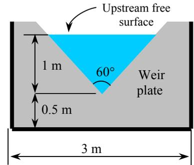
**13-110** The flow rate of water in an open channel is to be measured with a sharp-crested triangular weir. For a given flow depth upstream the weir, the flow rate is to be determined.  $\sqrt{EES}$
