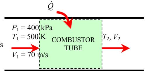
**12-103** Fuel is burned in a rectangular duct with compressed air. For specified heat transfer, the exit temperature and Mach number are to be determined.
