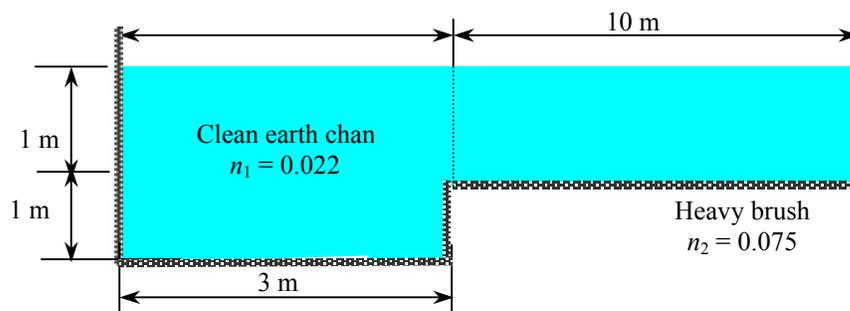
**Assumptions** 1 The flow is steady and uniform. 2 The bottom slope is constant. 3 The Manning coefficients do not vary along the channel.
