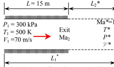
**Assumptions 1** The assumptions associated with Fanno flow (i.e., steady, frictional flow of an ideal gas with constant properties through a constant cross-sectional area adiabatic duct) are valid. **2** The friction factor is constant along the duct.
