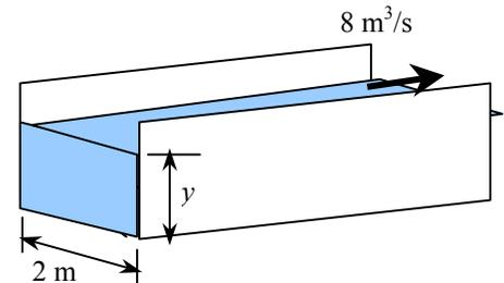
Therefore, flow is **supercritical** for  $y < 1.18 \text{ m}$ .
