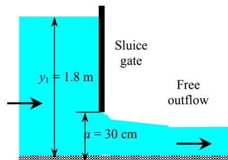
**13-135** Water at a specified depth and velocity undergoes a hydraulic jump. The fraction of mechanical energy dissipated is to be determined.
