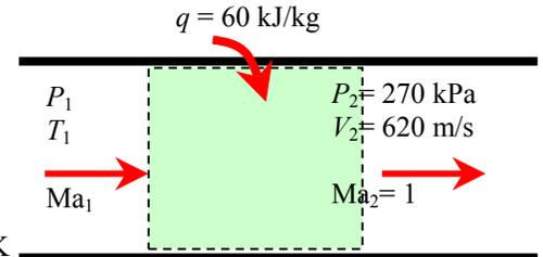
The inlet stagnation temperature is, from the energy equation  $q = c_p(T_{02} - T_{01})$ ,
