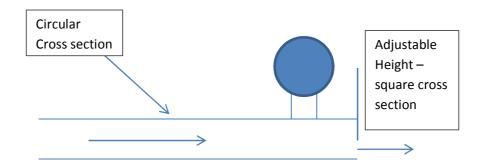
So the problem with our current setup is that we have no way of determining the pressure inside the pipe, we need some way to vary the velocity other than the flow. The setup above goes from a circular pipe to a square pipe with a adjustable height gate. This way we can vary the velocity and know both of them from the mass conservation equation as:
