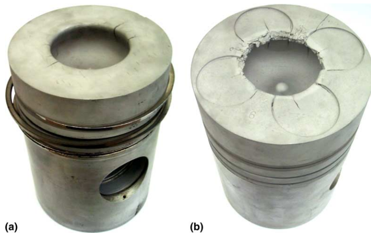
Fig. 11. Train engine pistons with damaged head: (a) piston 1; (b) piston 2.
