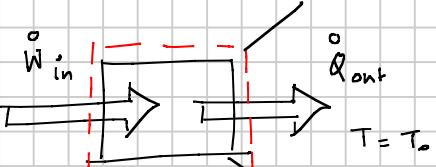
$$\text{Energy: } \frac{dE}{dt} \xrightarrow{\text{steady state}} = \sum_i \dot{m}_i \dot{j}_i - \sum_{\text{mech}} \dot{W} + \dot{Q} - \dot{W}_{ext}$$
